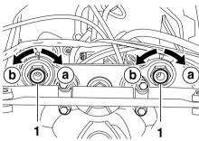
1. Spring preload adjusting bolt
