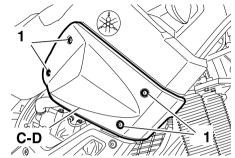
1. Panel mounting bolt C. Right panel D. Left panel
