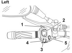
1. Pass switch "≣D" 2. Dimmer switch "≣D/ ≣D"
