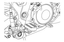
The operation of the brake pedal should be checked before each ride, and the pedal pivot should be lubricated if necessary.
