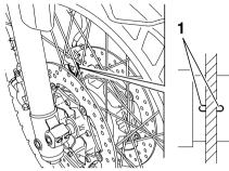
1. Front brake pad wear indicator groove
