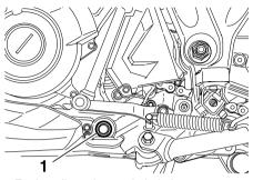
1. Engine oil crankcase drain bolt
