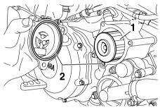
1. Engine oil filter element 2. O-rings
