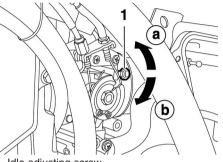
1. Idle adjusting screw a. Increasing the engine idling speed
