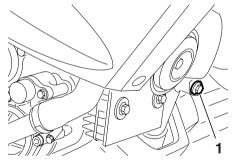
1. Engine oil tank drain bolt
