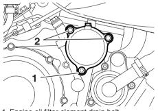
1. Engine oil filter element drain bolt 2. Oil filter element cover bolts
