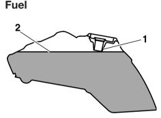
1. Fuel tank filler tube 2. Fuel level
