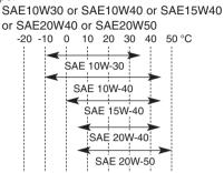
Recommended engine oil grade: API service SE, SF, SG type or higher Engine oil quantity:
