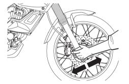
1. Place a stand under the engine to raise the front wheel off the ground.
